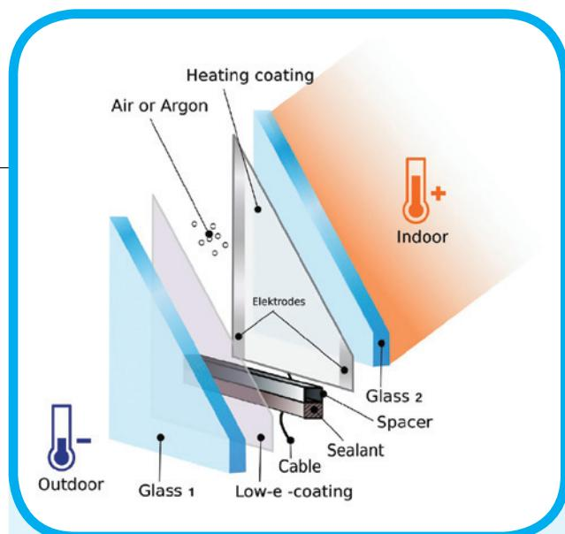
There are no wires criss-crossing glass. Instead, electricity is conducted via a low-E coating. The only way to tell that the glass is electrically heated is that it is always clear, even in cold climates. This example shows a double-glazed window, however, triple-glazing is predominant in Finland
