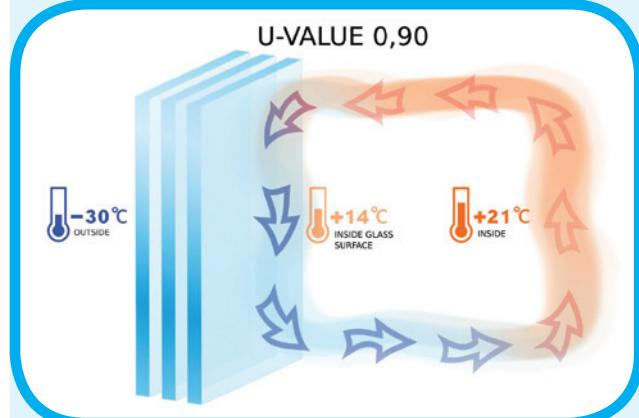
Convection is caused by the air temperature close to the window being lower than in the room. Cold air descends, moves across the floor and rises back up, causing a sensation of draft and cold radiation. When glass is heated just one or two degrees higher than room temperature, it stops convection and draft
